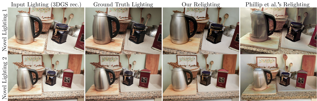
Figure 10: Qualitative comparison on real scene KETTLE. From left to right, from the same viewpoint: input lighting condition (view reconstructed using 3D Gaussian Splatting), target lighting, our relighting, Philip et al. [PMGD21] relighting. Top and bottom rows are two different lighting conditions. Philip et al. [PMGD21] exhibits much more geometry and shading artifacts compared to our method; in particular imprecise MVS preprocessing results in missing geometry.
