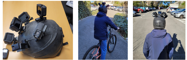
Fig. 9. Left: Our 6-GoPro HERO6 camera helmet rig. Middle: We performed captures on foot and (Right) on a bicycle at 6–7 km/h.
