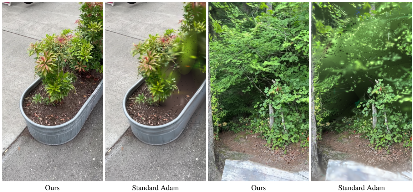
Figure 8: Standard Adam updates all parameters on every iteration irrespectively of whether their contribution to the rendered image, leading to divergence, particularly in cases when the primitives are obscured, or when they have many keyframes.
