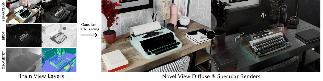
Fig. 2. Our method takes as input several buffers for every training view (left), and reconstructs a unique gaussian-based scene where reflections in novel views are computed with cached diffuse (middle) and physics-based path tracing (right). This figure shows ground truth input buffers from a synthetic scene, from top to bottom: separated targets (diffuse and non-diffuse), BRDF parameters (base reflectance and roughness), and geometry (depth and normals).
