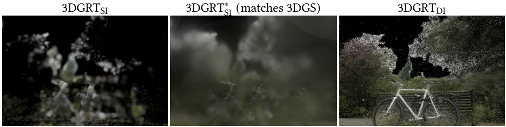
Fig. 3. Different Gaussian initializations visualized with 3DGRT. From left to right: sparse (SfM) initialization, sparse initialization with Gaussian scales matching 3DGS exactly (note how primitives are very large, which is unfavorable for ray-tracing), and dense initialization.
