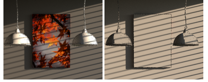
Figure 3: Visualization of outgoing radiance (left) vs incoming radiance (right). Since incoming radiance is a spherical function, we visualized \int_{\Omega} L_i(\mathbf{x}, \omega_i) d\omega_i . The incoming radiance is much smoother than the outgoing radiance.
